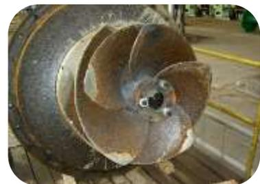
*Impeller for a large water pump has become badly eroded and required resurfacing. The impeller was abrasive blast cleaned and 2 x coats of 202 Ceramic Repair Fluid applied to the surface*
