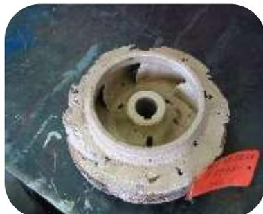
*Impeller from a sea water pump was badly eroded. The pump was obsolete and no spare parts were available. The surface of the impeller was rebuilt using 301 Epoxy Resin with glass fillers and then machined to a smooth finish. Once cured 2 coats of 202 Ceramic Repair Fluid was applied to all of the impeller to complete the repair*
