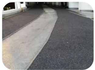
Resichem 507 DWPU was chosen as a ferry deck anti-slip coating system. Surfaces were mechanically abraded and degreased to remove all surface contaminants.
