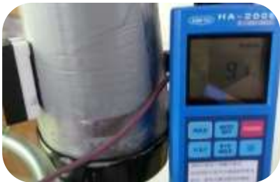
Container A was coated with 3mm of 560 Thermal Barrier XF. The surface temperature of the container increased to 9.1°C
