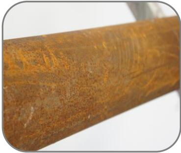
Surface of the pipe is badly corroded and pitted
